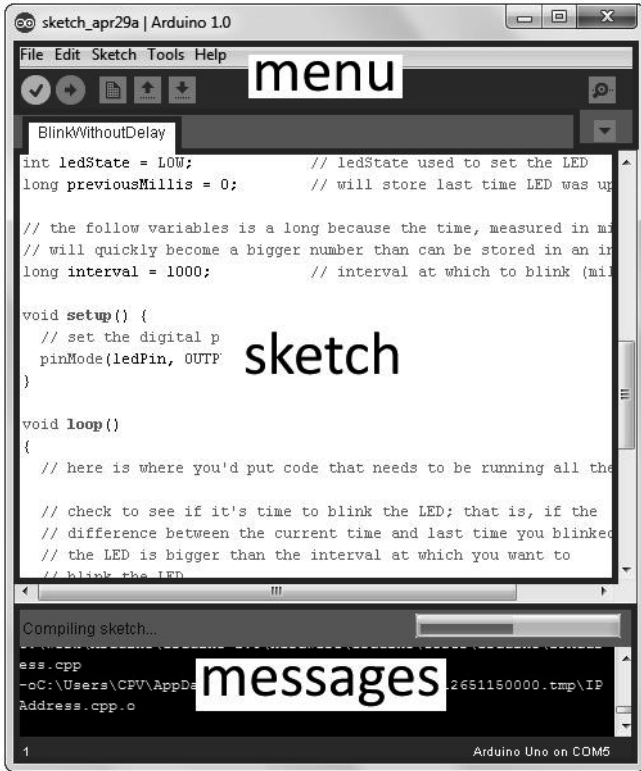
Figure 4-7 - The Arduino IDE and its three main areas.
