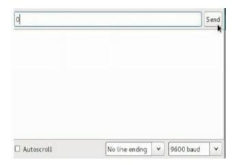
• In this example, we have used the *Serial.Read()*; instruction to read the data that was sent from the computer to the Arduino through USB, also we added the variable "value" to store the data.
