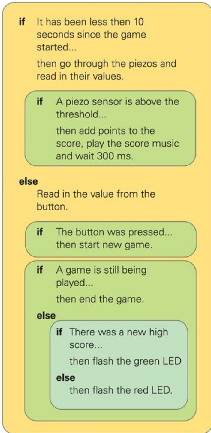
Figure 9-9 How a loop() works
