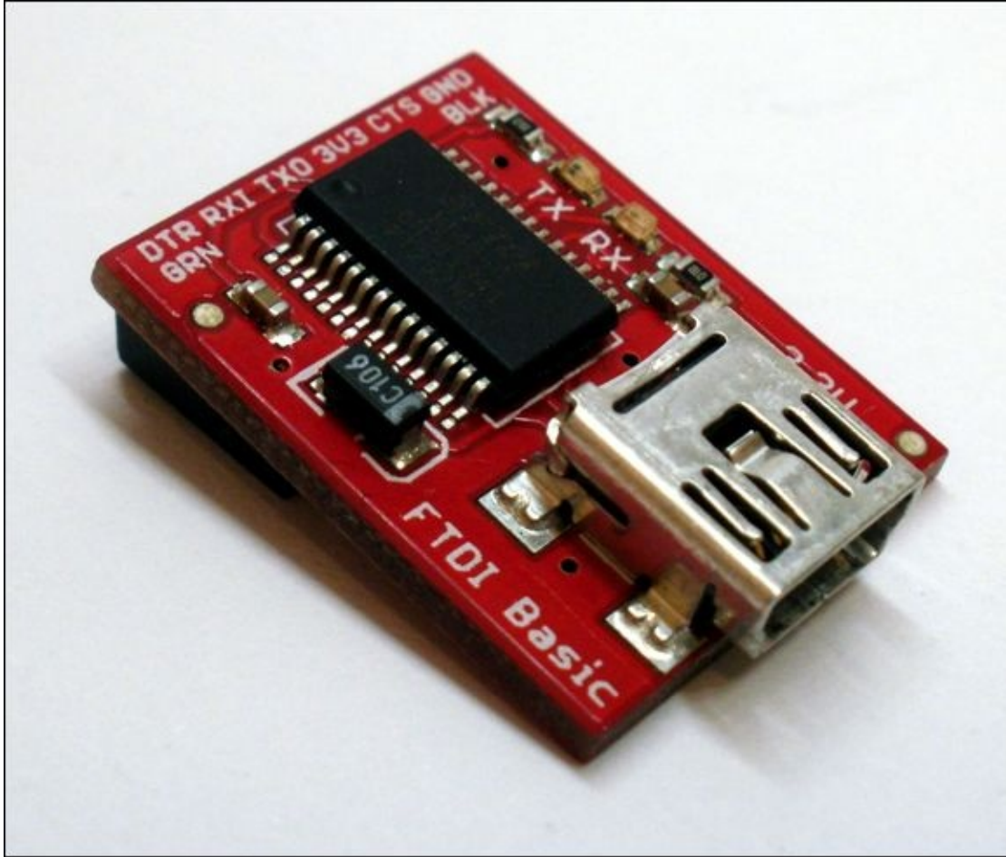
Figure 8-3 An FTDI programming board, which you need if you are using a type of Lilypad Arduino other than a Lilypad Arduino USB
