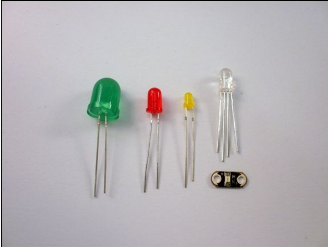
FIGURE I-5 Different types of LED, with a colour-changing LED on the right and below it a LilyPad LED
