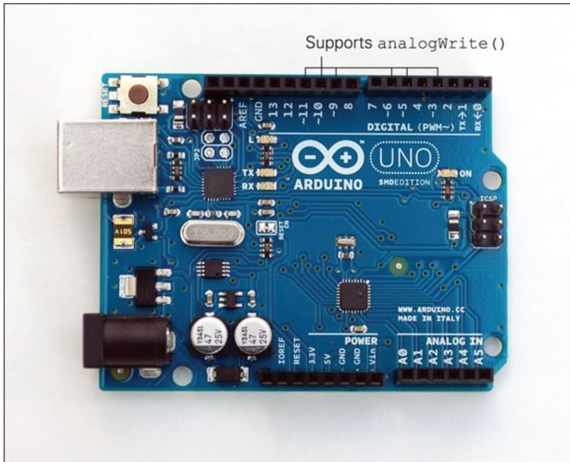
Figure 6-3 The pins that support analogWrite()
