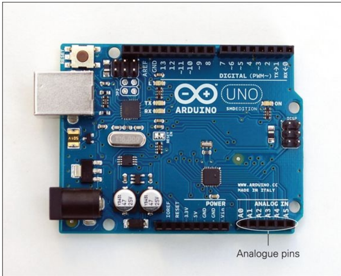
FIGURE 2-6 Analogue pins on the Arduino Uno
