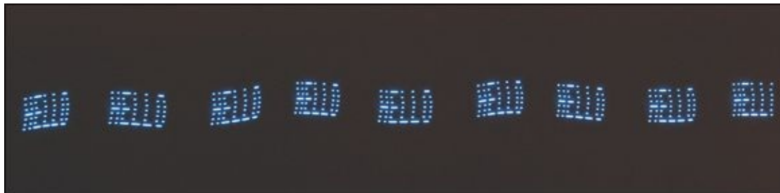
Figure 8-16 Persistence of vision message captured with a long-exposure photograph
