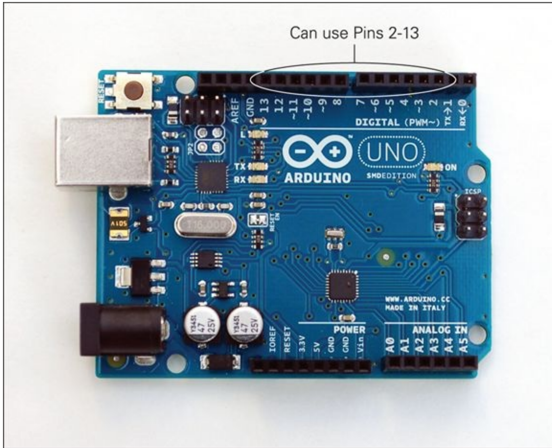
FIGURE 1-17 The digital pins on the Arduino board. Digital Pins 0 and 1 are special pins that you learn about later.
