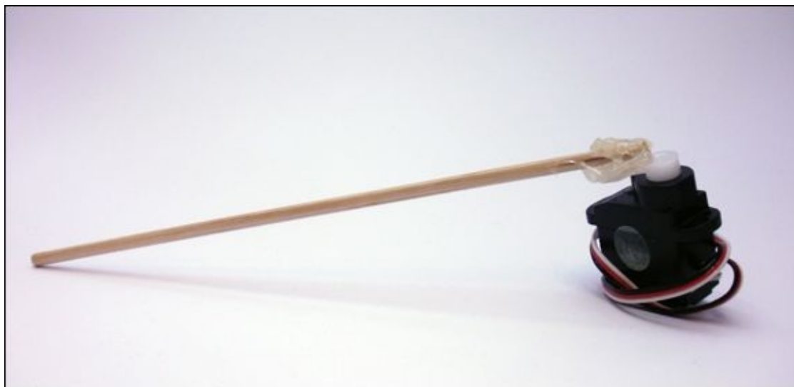
FIGURE 3-14 Extend the servo's arm by attaching an object like a paperclip or bamboo skewer.
