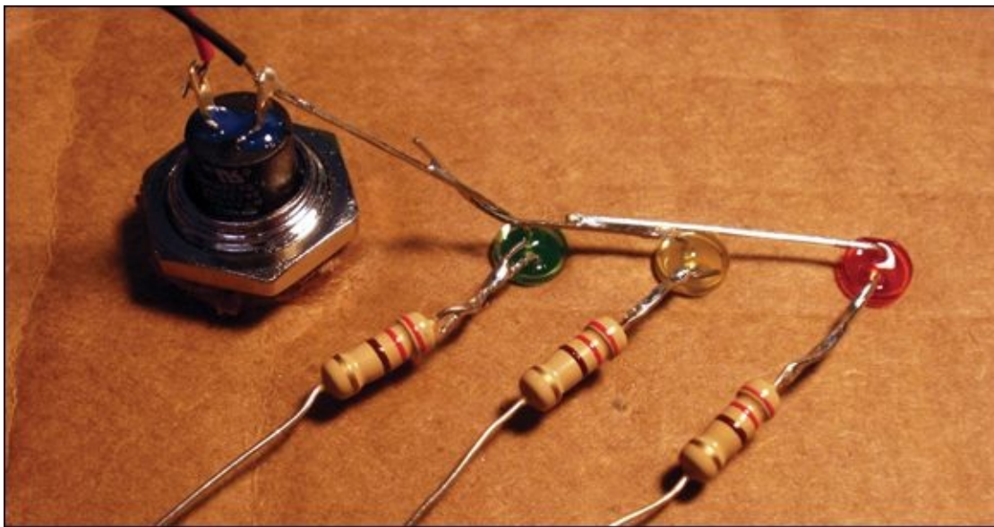
Figure 9-14 Solder the negative legs of the LEDs and one contact of the button together.
