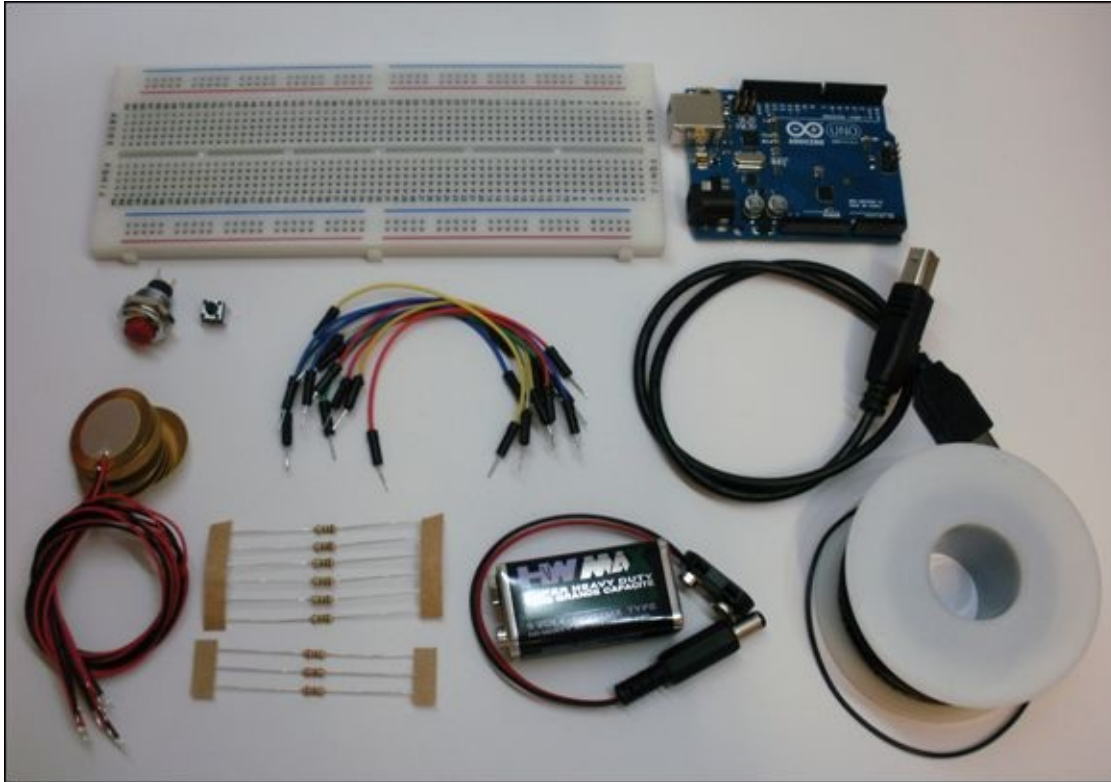
Figure 9-2 The electronic components you need to build your maze game
