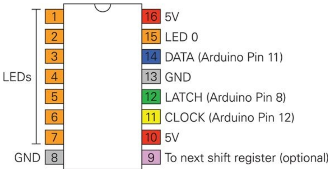
FIGURE 4-6 Pin-out diagram for the shift register
